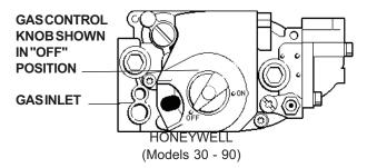
Fig. 29: Honeywell Gas Valve
